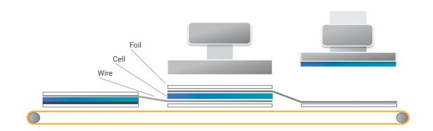
A 60 cell solar matrix is created by alternating 6 strings of 10 cells. The matrix is covered with encapsulant then placed between a sheet of glass and a backsheet.
